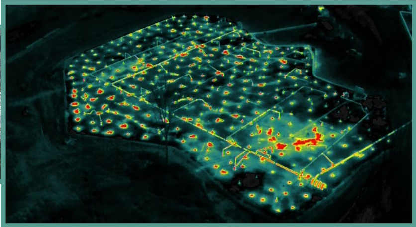
Burn Pit wellfield layout and corresponding thermal imaging of the wellfield during thermal treatment operations in October 2024.
